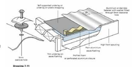
5 mm barrier of inert non-absorbent, non-reactive material. Alternatively self-supporting underlay may be used. Plastic strapping can be used for supported underlays, stapled with stainless steel staples to the vertical face of the purlins.
