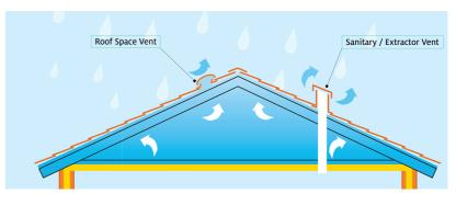
other is a sanitary vent cap which allows vent pipes from toilets and also from bathrooms, laundries and kitchens to exit straight up and out of the roof where natural air movement is at a maximum, to remove steam etc with no mechanical ventilation or less than required with the common horizontal venting.
