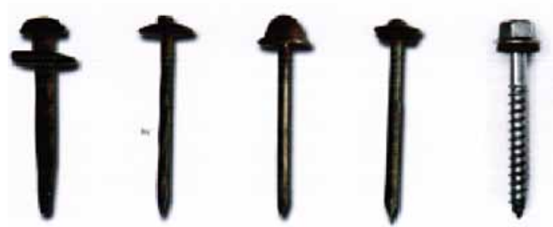
The evolution of roof cladding fasteners. From left: Hand-forged chisel-point nail with lead washer circa 1840; spring head, (the farmers' friend); lead-head; spiral shank; self-drilling Type 17 screw.
