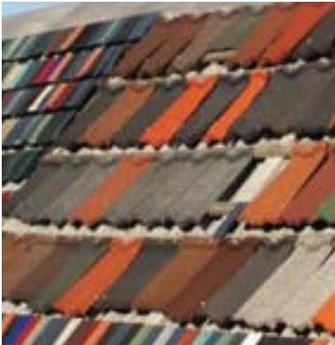
Extensive coatings test facilities in many locations provide a data base to improve paint systems
